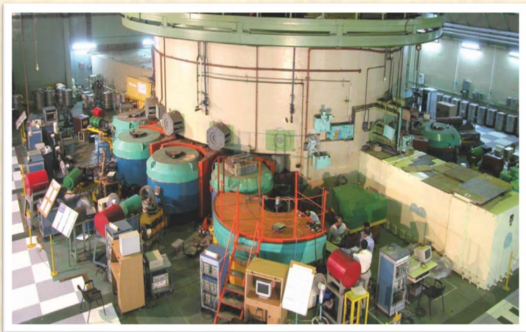
Steady State Superconducting Tokamak (SST-1) at IPR
